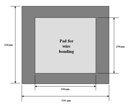
WaferArray: Saw step size is 590um x 490um
